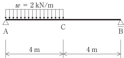
1.  $M = 8 \text{ kN} \cdot \text{m}$      $Q = 2 \text{ kN}$
